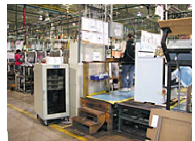
Range testing station at Whirlpool plant in Tulsa, Okla. Remotely operated Associated Research testing equipment is enclosed in cabinet at lower left.
